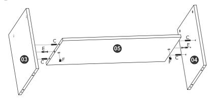
• Connect the Shelf (05) into the Left Side Panel (03) and Partition (04) using dowels (C) and the Minifix hardware (E + F).
