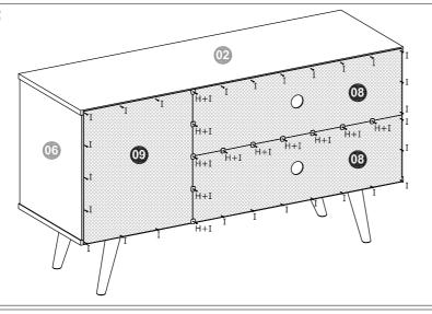
• Connect Back Panels (08) and (09) with nails (I). At the joining surfaces, use metallic plates (H) and nails (I).
