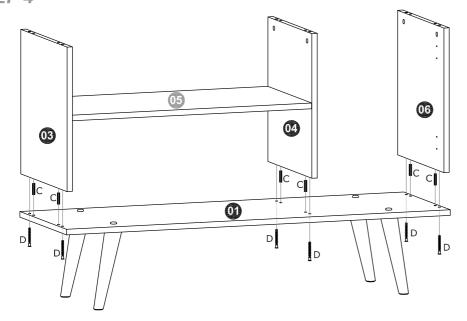
• Connect Side Panels (03) and (06) and Partition (04) into the Base (01) with dowels (C) and bolts (D).
